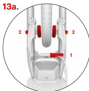
Adjusting the rear brake (V-brake)
