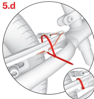
Fasten the end of the brake cable in the lock and secure with the cable tie, then trim the tie.
