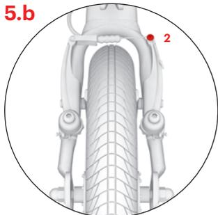
Check that the pads make enough space (1–2 mm) after releasing the brake levers. The distance can be adjusted by tightening or loosening the brake cable at the anchor screw (2).
