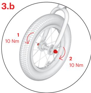
Place the wheel into the front fork so that is well-centered and tighten the nuts (1, 2). (For easier installation you can turn the balance bike upside down).
