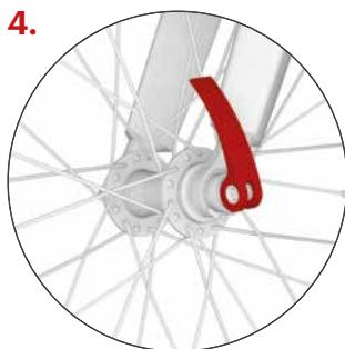
Tighten the adjustment nut of the quick release mechanism to the correct position. When it is in the correct position you will feel a noticeable resistance just before you close the mechanism completely. Close the quick release lever in a position so it does not touch the fork and simultaneously it cannot be opened accidentally while riding.
