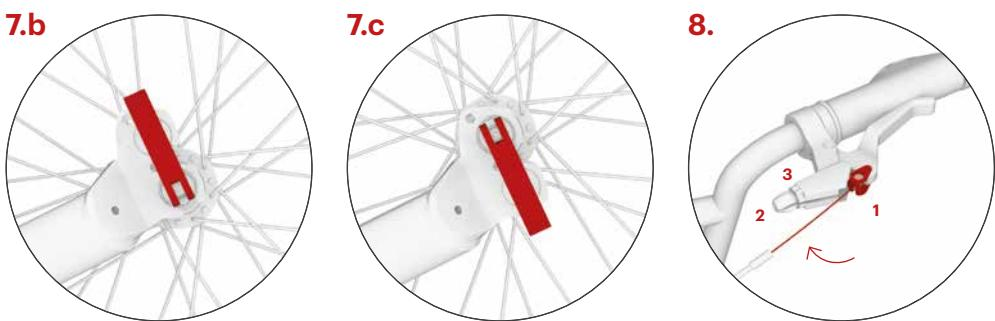
Two-position rear fork enables you to adjust the height of the footrest above the ground. Use the lower position for riding over rough terrain. Close the quick release lever. It should point upwards.
