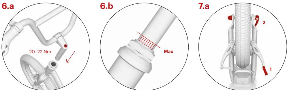
Insert the stem into the frame tube of the scooter and adjust the handlebar height taking care not to position it above the marked line, see pic. 6.b. Make sure that the handlebars are straight and then tighten the screw on the stem.
